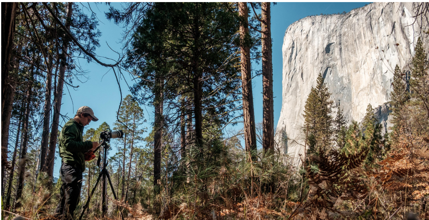
GIP intern Nikita Avdievitch conducting a “structure from motion” survey of the 2017 El Capitan rockfalls from the Yosemite Valley floor, Yosemite National Park, California. (NPS photo)
