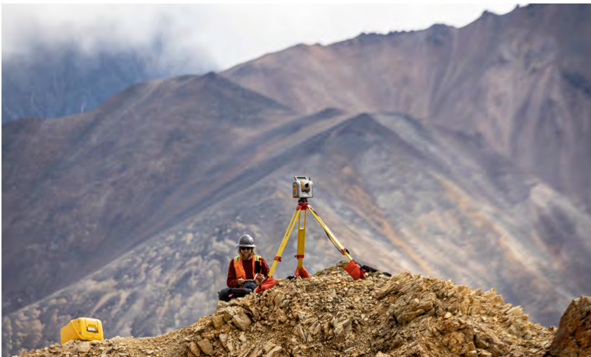
SIP Intern Loring Schaible setting up equipment to do a laser scan of the Pretty Rocks landslide in Denali National Park, Alaska (NPS photo).
