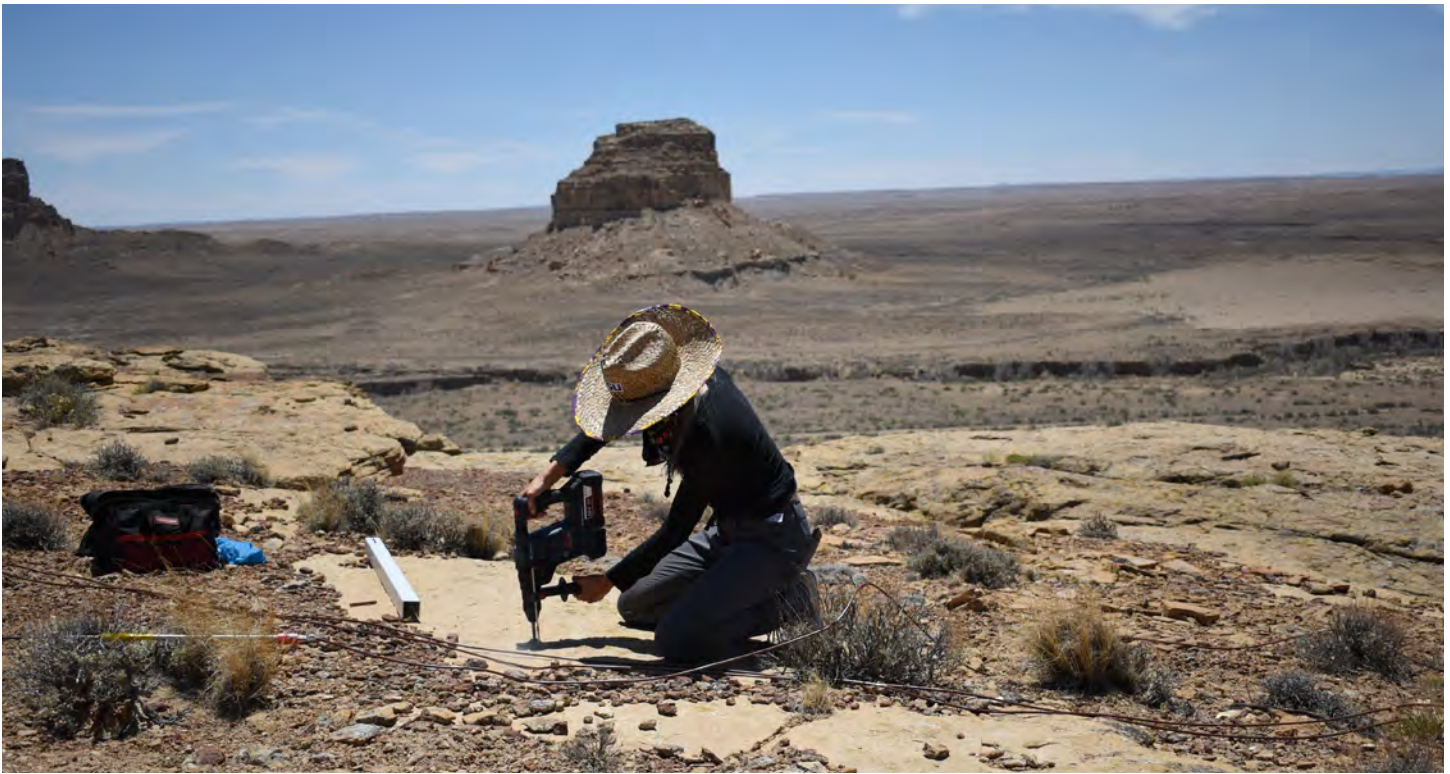
SIP Intern Anna Sivils drilling into sandstone for vibrating wire sensor installation at Chaco Culture National Historical Park, New Mexico. (NPS photo)
